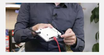
Use the EBS Power Supply to provide the Base Station with 6V power. You can use the EBS Ethernet cable to connect the Base Station to your existing network.
