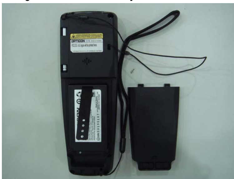
Figure 2-3. Insert the battery pack
