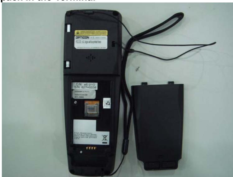
Figure 2-2. Detach the battery cover from Terminal
