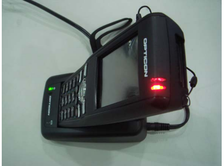
Figure 2-5. Charging Terminal with CRD-15 cradle
