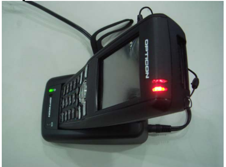
Figure 2-6. Charging Spare Battery with CRD-15 cradle
